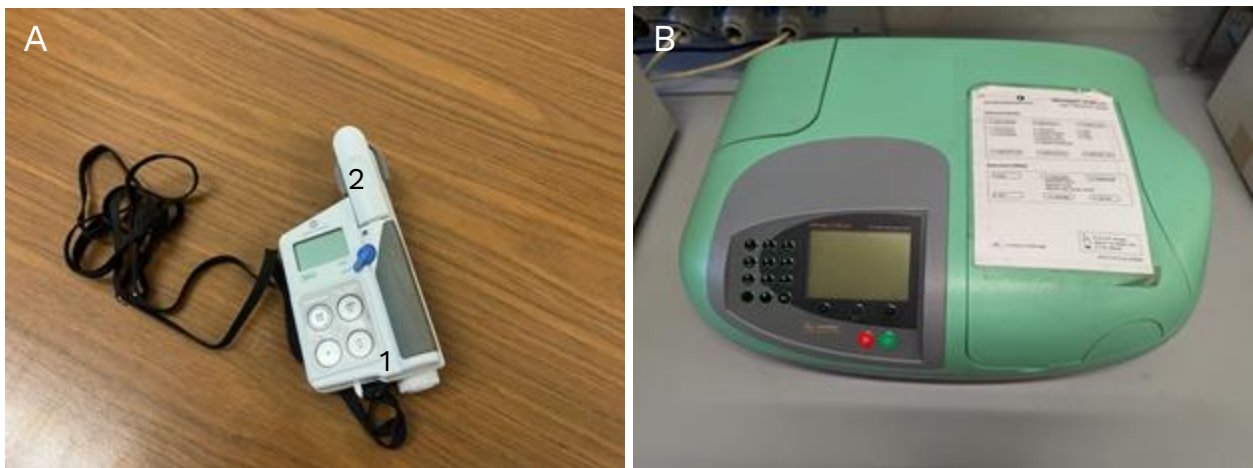
Figure 3. Devices for measuring leaf chlorophyll concentrations (A) SPAD-502Plus chlorophyll meter (Konica-Minolta, Tokyo, Japan). 1 – Power-and-Control-Unit 2 – Clip on sensor. (B) Spectrophotometer (Ultrospec™ 2100 pro, GE Life Sciences, Buckinghamshire, UK)
