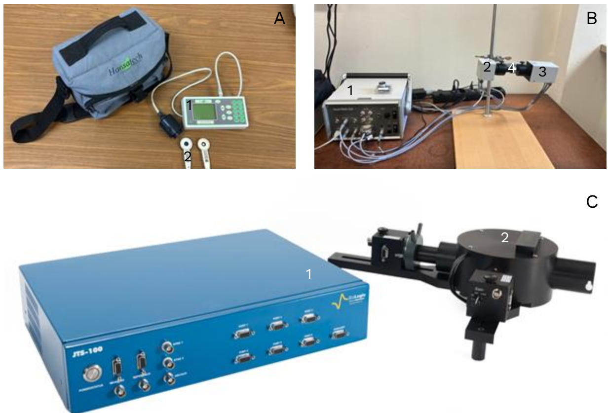
Figure 2. Devices for characterization of photosynthetic performance (A) Handy-PEA+ (Hansatech-instruments). 1 – Control unit and sensor; 2 – Leafclips. (B) DUAL-PAM-100 (Walz, Effeltrich, Germany).
