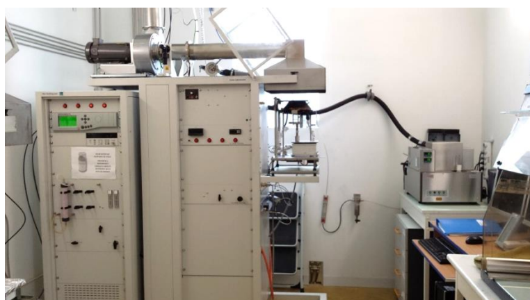
Figure 12. Cone calorimeter (FTT, UK)
